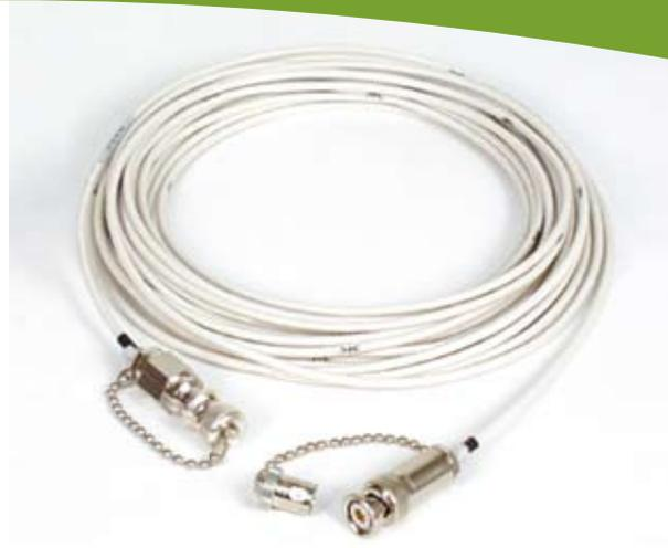
Triaxial BNC (bayonet) connectors are the 2-slot/lug, 1/4-turn locking type. The male connector has a pin insert and is always accompanied by a ferrule with locking slots. It is available only for cable mounting. The female connector has a socket insert and locking lugs that mate with the ferrule. It is available for cable mounting or panel (bulkhead) mounting, with either flange or threaded mounting.
