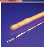
MOSFET dosimeters are small, light-weight, unobtrusive, and versatile. Pictures above show the small size of the microMOSFET, a high-sensitivity MOSFET being used to measure scatter dose to the thyroid, and the Linear sive Array for use in brachytherapy.
