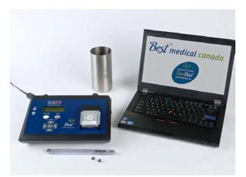
The VALIDATOR system, which uses electronic MOSFET dosimeters, is versatile and allows real-time dose readout and verification for radioisotope, X-Ray or linear accelerator based irradiators, used in hospitals, blood banks and clinical research laboratories.
