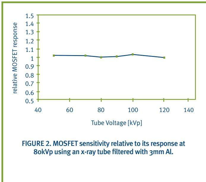
FIGURE 2. MOSFET sensitivity relative to its response at 80kVp using an x-ray tube filtered with 3mm Al.
