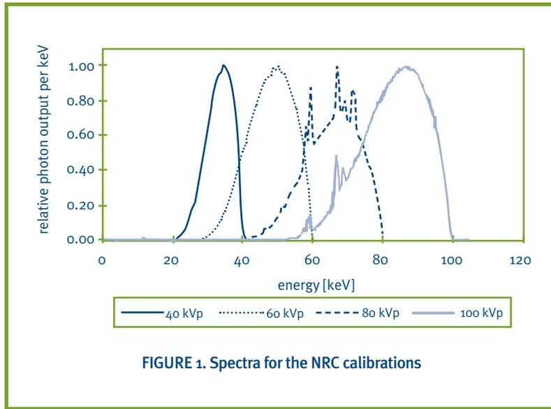
FIGURE 1. Spectra for the NRC calibrations
